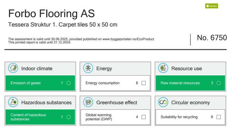
Manufacturer: Forbo Flooring AS Generic product: Carpet Product group: Flooring Assumed technical lifetime: 10 years Moisture resistance: Not affected Cleanability: Not applicable Reference value GWP: 8.3 kg/m<sup>2</sup> <sup>')</sup> Structure Components: 255 Floor Surface
