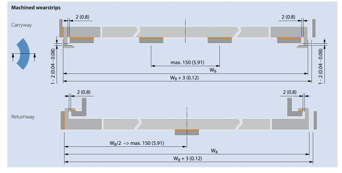
For a smooth run, especially for high curve radius compared to collapse factor ( $C_c$ ) of the belt, a support at the outside G-tab is possible.
