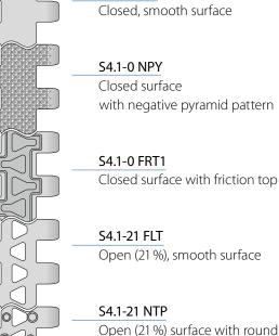
Open (21%) surface with round studs. Version available without round studs at the side (25 mm indent)
