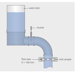
For this reason, Forbo Siegling has developed a drainage test for modular belts. The published "FLOW RATE" is defined in liters per second (I/s) and will support our customer when choosing the right belt for a water drainage application. (Custom testing with other fluids is possible.)
