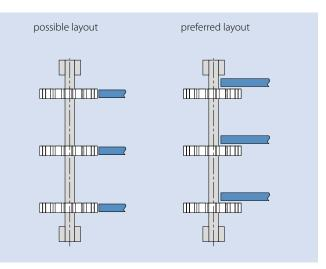
If wearstrips end at the sprocket edge, ensure a distance of  $X \le 1.5$  Pitch.
