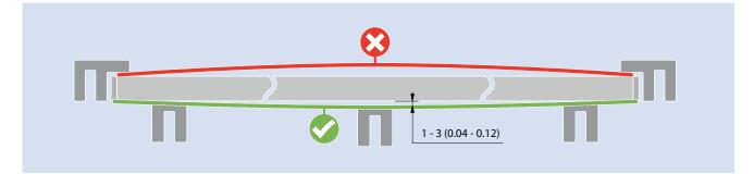
Series 5 and 9 are assembled with steel pins causing a higher stiffness. This reduces the tendency to belt lift in the first place and secondly makes the belt much more laterally stiff such that a lower positioned center wearstrip would not lead to a bow downwards but rather leave space between the wearstrip and belt.
