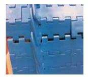
1 Move both belt ends until they interlink correctly
