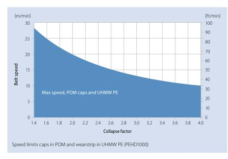
For radius conveyors running at higher speeds, Series 11 offers an alternative with caps or HD on the belt edge made of a special robust, resistant material identified by material code HW. For these we recommend using wearstrips in Nylatron NSM, a special PA material with solid lubricant additives. This material combination will in general offer an extended service life for conveyors with heavy loads or conveyors running in abrasive environments.
