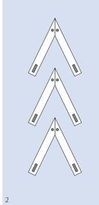
Thermal expansion and contraction must be taken into consideration when mounting the support. These effects can be absorbed by slots and appropriate distancing between the wearstrips (see calculation in "Effect of temperature" in <u>chapter 4.4</u>). The admissible temperature ranges, as given by the manufacturer, must also correspond to the expected operating conditions.
