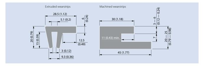
Dimensions in mm and inches (in). All imperial dimensions (inches) are rounded off.
