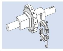
Siegling Prolink Retainer Rings provides a quick, easy and reliable solution for fixing the sprocket (see <u>page I-216</u> for details).
