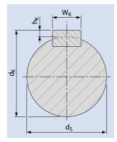
Shaft dimensions (round and square) according to ISO 286-2 h12 (or closer degree of tolerance e.g. h7) can be used.
