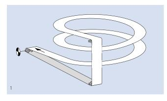
Example of declined conveying to join two production units with different heights (1).
