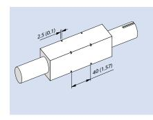
Shaft 40 x 40 mm. Fastening the sprocket with a retainer ring in accordance with DIN 471 (Seeger circlip ring), d = 56 mm. Detailed dimensions are to be found in appendix on <u>page VI-11</u>.
