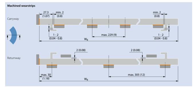
For a smooth run, especially for high curve radius compared to collapse factor ( $C_c$ ) of the belt, a support at the outside G-tab is possible.
