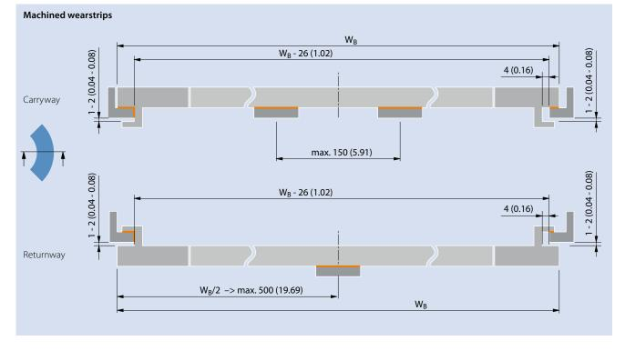
For a smooth run, especially for high curve radius compared to collapse factor ( $C_c$ ) of the belt, a support at the outside RG-tab is possible.
