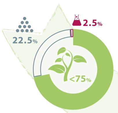
The proportion of renewable raw materials is up to 75 %. The main components are linseed oil, natural resin, wood flour and jute.
