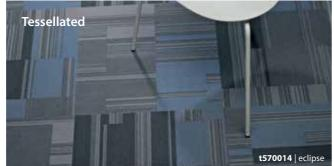
Flotex tiles meet the requirements of EN 1307 Description Flocked flooring ISO 1765 Total thickness 5.3mm 50cm x 50cm. Tiles per box: 12 (3 m<sup>2</sup>) Tile dimensions 60 x 60cm & 100 x 100cm available on request Collection size 10 Application EN685 Class 33 heavy Total weight 5.4 kg/m<sup>2</sup> Absasion resistance EN1307 annex F > 1000 cycles Slip resistance Pendulum test DRY - very low slip risk. WET - Low slip risk EN-ISO 717-2 Impact sound  $\Delta Lw = 19 \text{ dB}$
