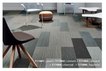
Flotex seagrass meet the requirements of EN 1307 Description Flocked flooring Total thickness 5.3mm ISO 1765 Tile dimensions 100cm x 25cm. Tiles per box: 10 (2.5 m<sup>2</sup>) Collection size 6 Application EN685 Class 33 heavy Total weight 5.4 kg/m<sup>2</sup> Absasion resistance EN1307 annex F > 1000 cycles Slip resistance Pendulum test DRY - very low slip risk. WET - low slip risk EN-ISO 717-2 Impact sound  $\Delta Lw = 19 dB$ ISO 354 Sound absorption 0.10
