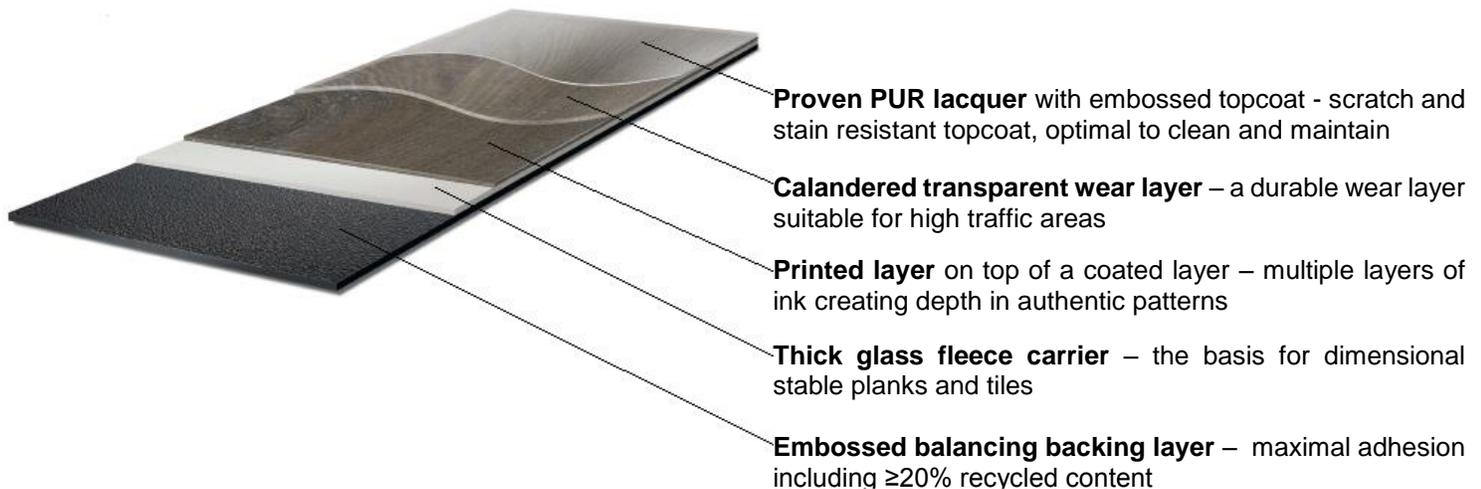
Figure 1: Typical construction
