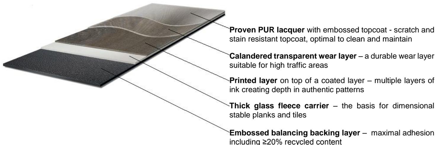
Figure 1: Typical construction
