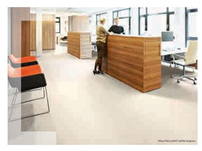
Allura Flex is a collection of high quality, dimensionally stable, heterogeneous loose lay vinyl tiles and planks which are adhered with tackifier rather than permanent adhesive.
