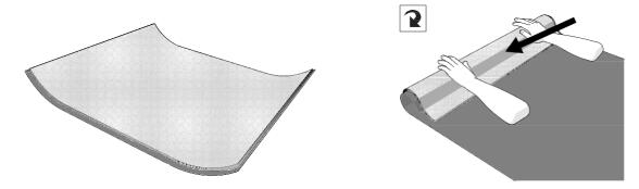
There is an arrow indicating pile direction on the reverse of every backed sheet product. Install sheets with arrows running in the same direction.
