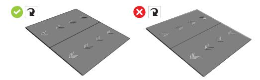
For all Coral textile products (except Coral duo) with an Everfort vinyl backing, trim with a straightedges and knife from the back of the sheet. Remove the 2.5cm edge border plus an additional 1cm to provide a suitable edge for butt jointing. Do we have a preferred direction for laying in relation to traffic flow?
