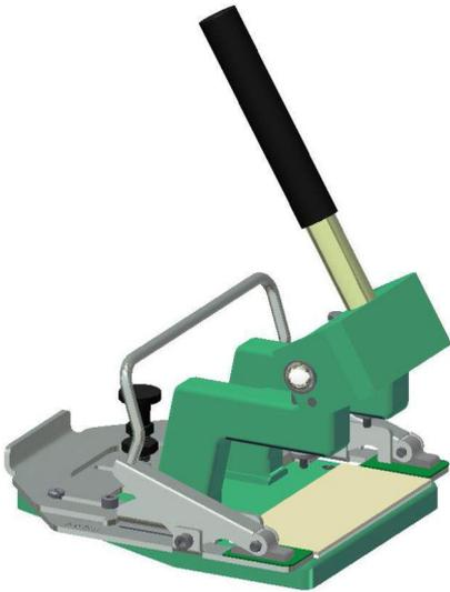
Punching presses of the PP-ZP-V/40-3 type are used to prepare Z-splices for belt widths up to 40 mm. Splices 35, 75 and 110 mm in length can be punched symmetrically. The adjustable that can be set to punch symmetrically is included in the scope of delivery. Without punching set!
