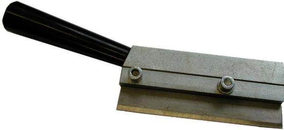
Handy device to prepare the punch-cutting for the Z-splice of the belt material.
