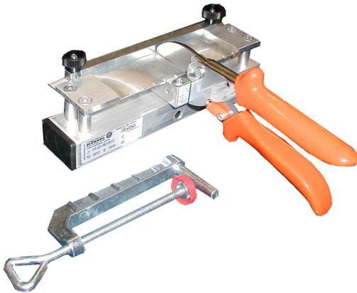
Hand-Z-shears of the PP-ZC-35/120-3 type are small tools for preparing Z-splices, used for fabricating Forbo Siegling belting material.
