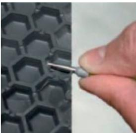
The connection to the tile can be made with a self-adhesive copper tape (or conventional grounding cable).
