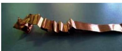
Another method of earthing is to use crimped copper tape under the tiles to ensure a good connection to the underside of the Colorex Plus tiles.
