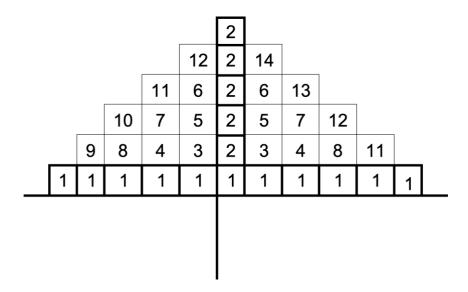
Lay subsequent tiles outward from either side of the centre start line forming a pyramid as per the diagram above. Locate the corner connectors of each tile and secure the connectors using a dead blow (non-rebound) hammer. Finish by hammering the remaining connectors on each side of the tile.
