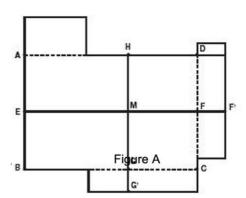
The centre line is drawn as follows: a chalk line is snapped from centre of wall A-B (=E) to the centre of wall C-D (=F). The centre of line E-F is found (M). Draw a perpendicular line through M using the 3:4:5 method to establish G-H (Figure A).
