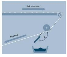
Scraper should lightly touch the belt on the return side just after product has been discharged. The angle "A" normally will be between 100 and 120 degrees.
