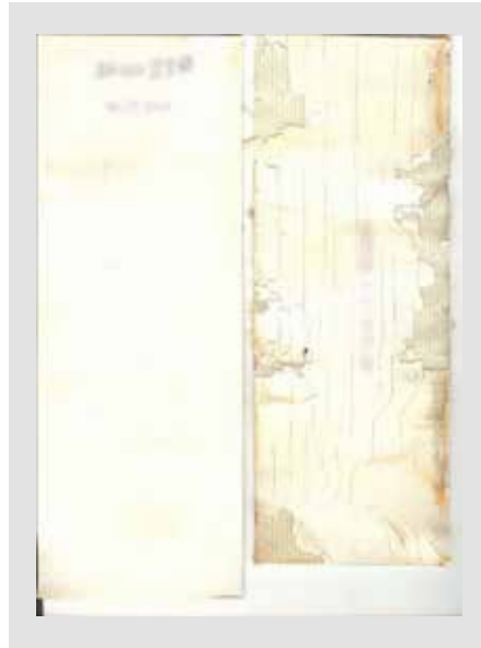
Fig. 4: Comparison of hydrolysis-resistant TPU and standard TPU after constant exposure to water, 100°C over a longer period of time (static)
