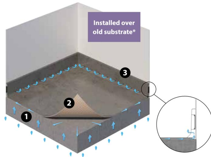
**1** Overclean protective finish for ease of cleaning and maintenance.
