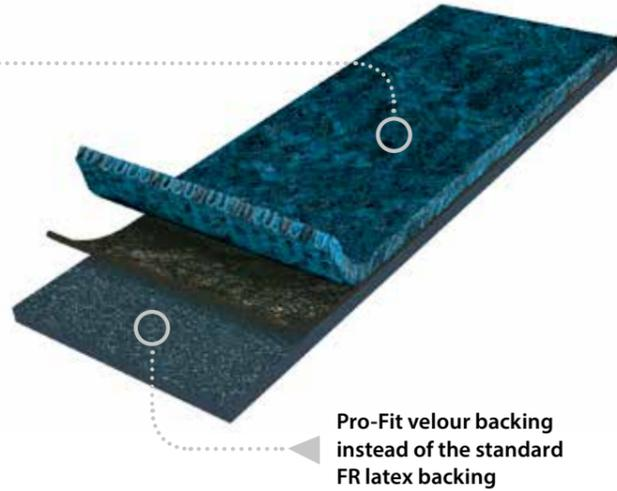
Customers who use this system experience far shorter first installation times (normal adhesive installations require 24 hours drying time). For renewals the advantages are even greater as it is simply 'pull up the old and drop down the new floor covering' that is required. No glue removal, no difficult sanding, no drying time.
