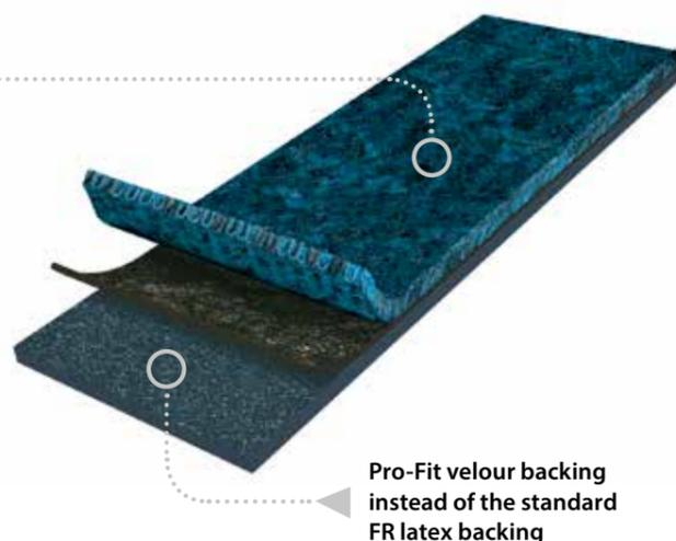
Customers who use this system experience far shorter first installation times (normal adhesive installations require 24 hours drying time). For renewals the advantages are even greater as it is simply 'pull up the old and drop down the new floor covering' that is required. No glue removal, no difficult sanding, no drying time.
