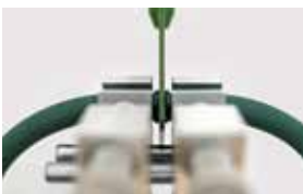
Melt the ends of the belt on the welding plate
