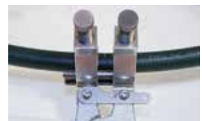
Insert the belt ends into the pliers and fix in place
