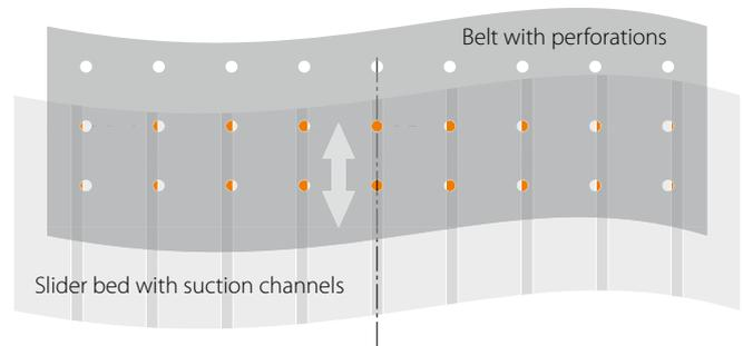
Fig. 1: Decreased suction cross section due to transverse contraction
