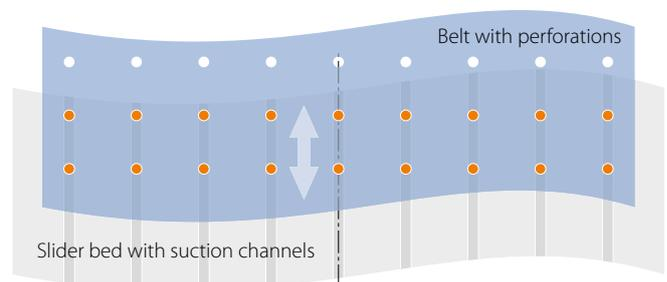
Fig. 3: Optimum suction cross section after belt tensioning because transverse contraction has been taken into account beforehand
