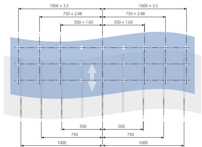
Fig. 2: Increase in the perforations' center distances during production (sizes serve as examples)
