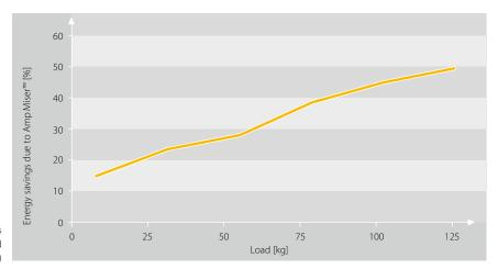
Energy savings depending on the load (test rig)
