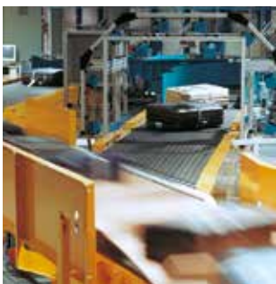
Perfect transfer of items conveyed due to small return radii; short take-up ranges thanks to the belts' tight length tolerances.
