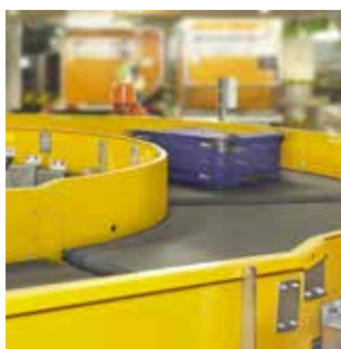
Reliable conveying due to a special fabric structure (distributing forces in the belt well).
