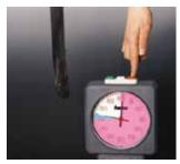
Flame-retardant belts cease to burn in seconds (green section) as soon as the gas flame is removed.
