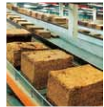
Conveying of bales: extreme punctual loads in stop-and-go operation.
