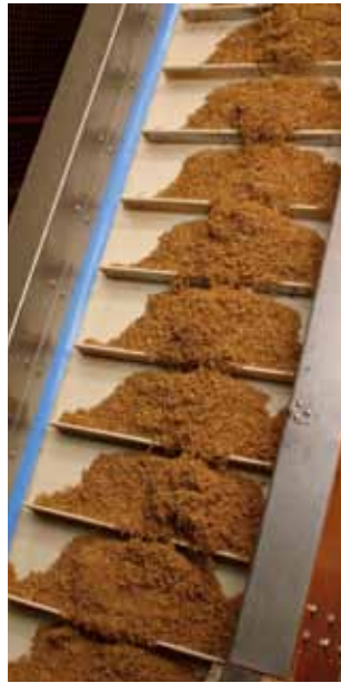
In many cases, conveyor belts equipped with profiles can replace conventional equipment with metal rakes, therefore reducing expensive set-up times.
