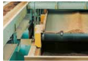
Horizontal conveying on a shuttle for the loading of the silo. The belt types with smooth surfaces used here can also be used for inclined conveying up to angles of about 20°.
