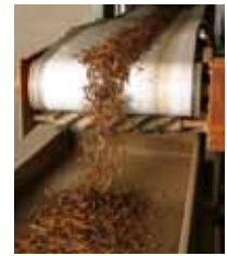
Conveying with a troughable belt.
