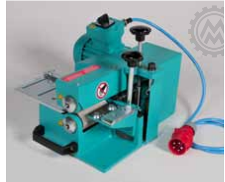
PS-PM-110/V; splitting and peeling machine
