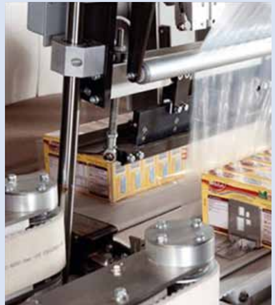
Siegling Proposition belts in a packaging machine.
