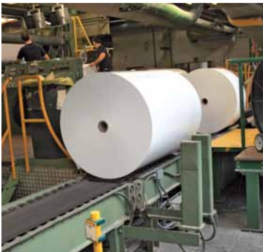
Siegling Transtex can easily handle punctual loads of 1500 kg without damaging the layers of paper on the outside.
