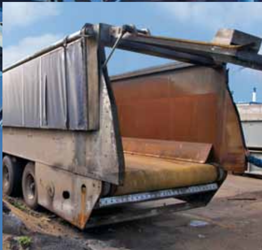
Unloading belt for 40 tons of hard coal. It took Siegling Transtex to make this compact conveyor design possible.
