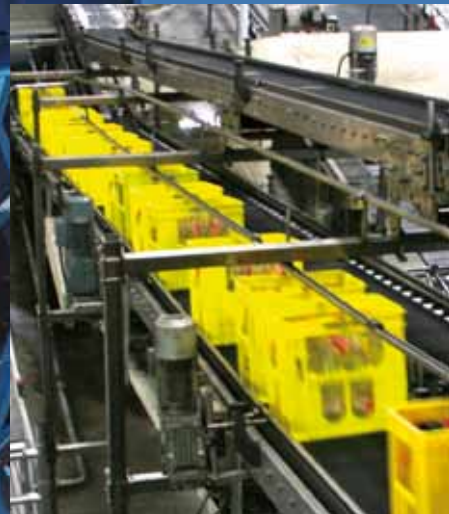
Large gradient angles can be achieved even for heavy-duty loads and when products conveyed are wet.
