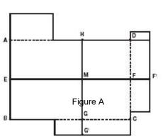
The centre line is drawn as follows: a chalk line is snapped from centre of wall A-B (=E) to the centre of wall C-D (=F). The centre of line E-F is found (M). Draw a perpendicular line through M using the 3:4:5 method to establish G-H (Figure A).
