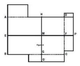
Starting at centre point M, measure out lengthwise and width wise to the walls. Wherever possible, cuts of less than 60mm or so should be avoided as these are more likely to come loose at some stage in the life of the installation. Adjust the position of lines E-F and G-H if necessary.
