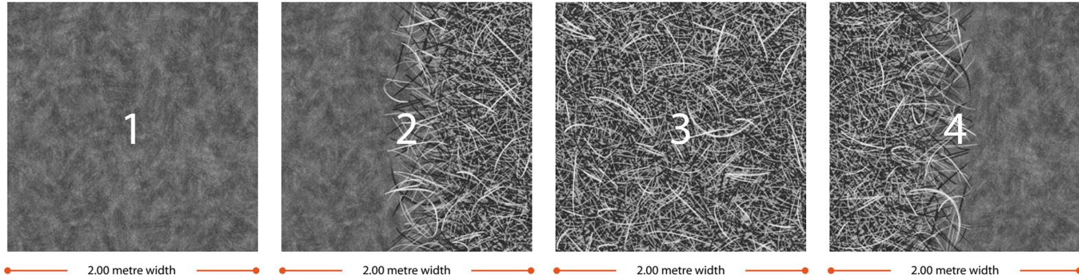
• To ensure full colour matching, Flotex sheets should be installed in the same direction. Make sure the arrows on the back of the sheet indicate the same direction.
