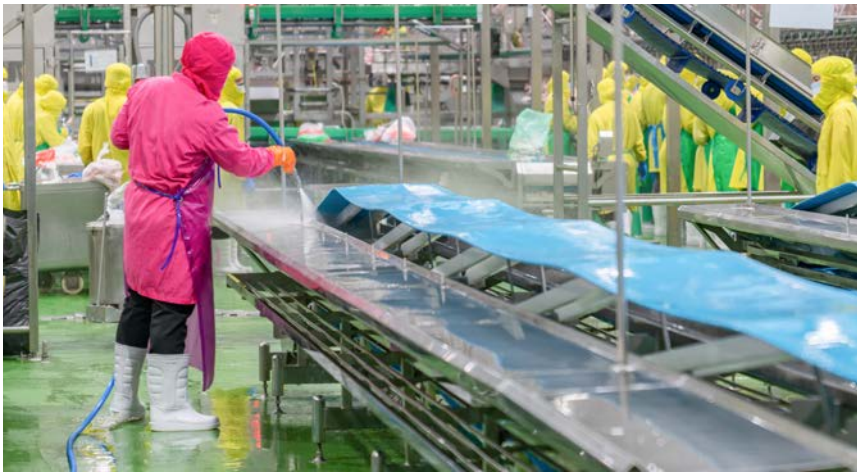
Fig. 4: Homogenous conveyor belt with quick tensioning device and lifting device.
