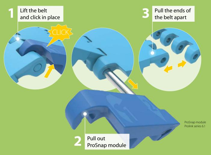
Several ProSnap modules can optionally also be fitted to the belt. This makes the distances covered to open the belt shorter and fitting easier. What's more, if a belt's damaged, a whole segment can be replaced quickly.
