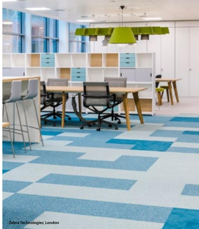
considerably to total sound absorption. The use of Flotex and Forbo carpet tiles reduced walking noise in a neighbouring room by up to two classes (10 dB). Resilient floors scored less impressive results of course, though Marmoleum was more effective than wood and stone, for example.
