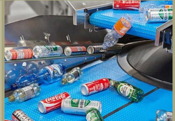
Prolink series 8.1 and 4.1 in polyoxymethylene (POM) fitted to market-leading, high-performance counting and sorting systems.
