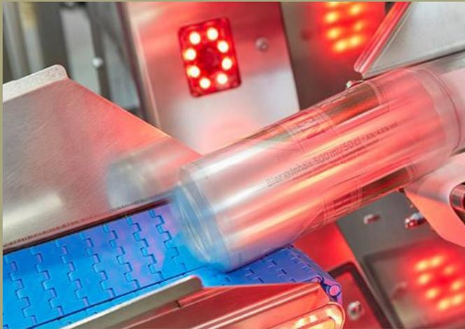
The HLZ MD Ultra has a scanner unit that registers the barcodes, matrix codes and security marks of the beverage containers passing through.
