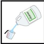
3. Make a cleaning solution by diluting a neutral pH cleaner in strict accordance with the manufacturer's recommendations. The pH of the cleaning solution must be between 6.0 – 8.0 pH.
