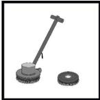
5. Scrub the floor with a 175 RPM floor machine using a flagged bristled brush such as a Malish nylon carpet shampoo brush #812915 or equivalent.
