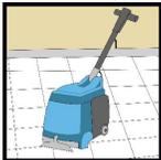
6. Use a self-contained portable extraction machine, preferably with counter-rotating brushes to extract the floor using clean water only. Set the brushes to ensure maximum agitation and contact with the fibers.
