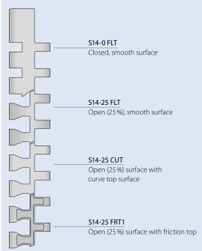
Sprockets and profiles available in different sizes and designs
