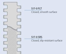
Sprockets and profiles available in different sizes and designs
