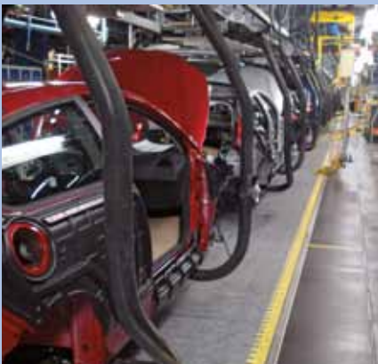
As worker belts in the automotive industry, Siegling Prolink modules are safe to stand on.
