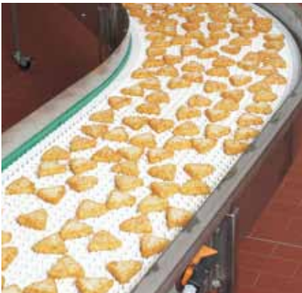
Siegling Prolink curved belts are ideal for space-saving drying or freezing.
