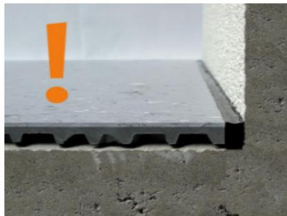
Wrong! A three-sided adhesion of PUR sealing compound inhibits free expansion and may lead to damages!
