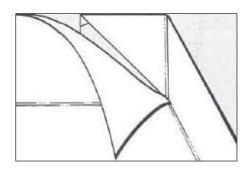
3. Cut the excess material to the 45 degree angle
