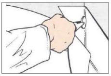
2. To enable the material to bend more easily, the reverse side of the insert should be grooved to approximately half thickness of the material using a 'P' Type grooving tool.
