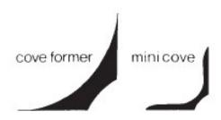
The following skirting details below show pencil cove (no cove former used) and all internal and external corners cut and heat welded at 45 degree angles. **Note:** All sheet joints must be heat welded.
