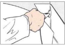
2. Press the floor covering into the corner with a roller
