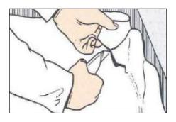
1. Fold the floor covering up to get 2 equal parts from each side of the wall. Cut in a line approximately 5mm off the floor, perpendicular to the fold. Fold up the floor covering against the wall. The gap must be filled in with an insert.
