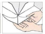
• Safestep should be rolled with a 3 wheeled 45 kg roller as soon as possible after laying and within the open time of the adhesive – the open time of the adhesive will depend on site conditions and porosity of the subfloor. Areas that cannot be rolled with the large roller e.g. abutments such as door frames or skirting boards should be rolled with a hand roller or pressed into the adhesive with a rubbing hammer.
