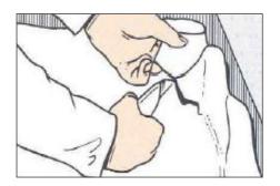
1. Cut the floor covering at a 45 degree angle approximately 5mm off the floor to make future welding easier.
