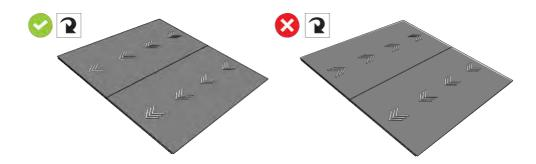
For all Coral textile products (except Coral duo) with an Everfort vinyl backing, trim with a straightedges and knife from the back of the sheet. Remove the 2.5cm edge border plus an additional 1cm to provide a suitable edge for butt jointing.
