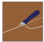
For a perfect finishing, trim off excess of welding rod in 2 steps.
