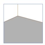
Subfloor has to be flat, permanently dry, solid and clean.
