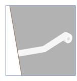
Install the modul'up adhesive tape (ref 792) on the subfloor at sheet seams and threshold lines.
