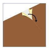
Remove the protective film from the adhesive tape (using a cutter blade for example).
