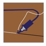
Groove first the seams. Then hot weld properly joins of Sarlon trafic modul'up.
