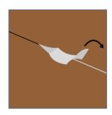
Go on removing the protective film over the lengths of sheets and smooth carefully the seams.
