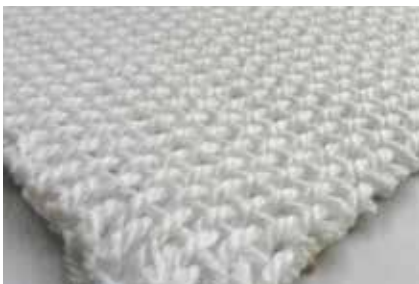
Multi-layer fabric used in Transtex types (interwoven fabric)
