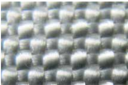
Fabric with plain weave Warp: Multifilament yarn Weft: Multifilament yarn
