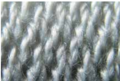
Fabric with 3/1 broken twill weave Warp: Staple fiber yarn Weft: Monofilament yarn smooth side
