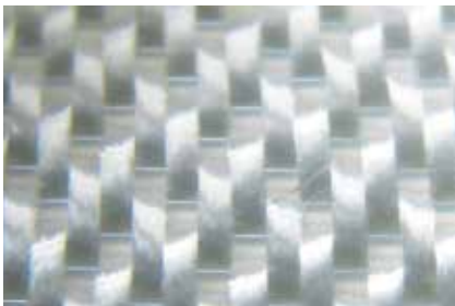
Fabric with 3/1 broken twill weave Warp: Multifilament yarn Weft: Monofilament yarn smooth side
