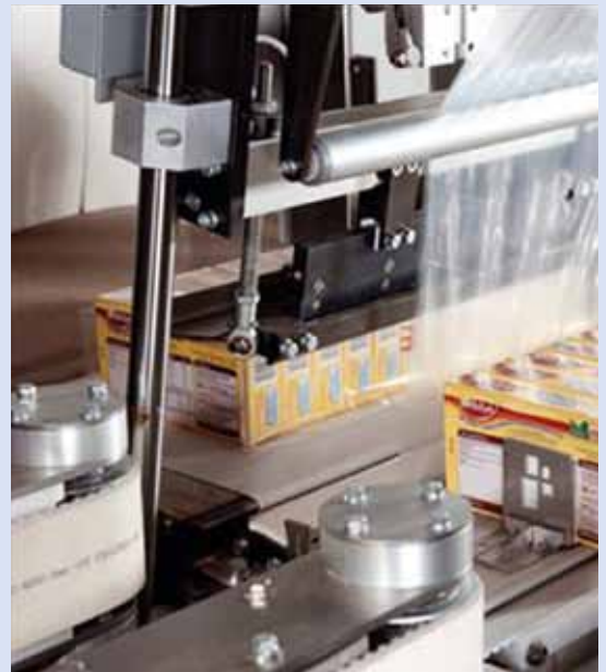
Siegling Proposition belts in a packaging machine.
