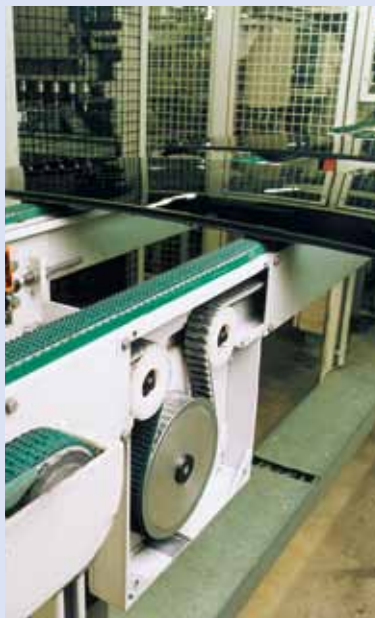
Conveying of car windows by belts running synchronously. The coverings on the reverse face of the timing belts treat the goods gently and improve the grip.
