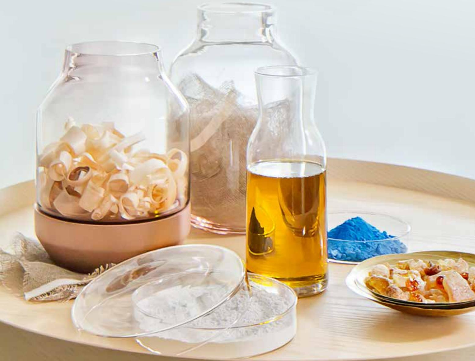
Marmoleum Click is a flooring product made primarily from renewable natural resources. The top layer is linoleum, a bio-based, ecologically produced material made from 97% natural raw materials, 70% of which are rapidly renewable, like flax (linseed) and wood flour, along with 43% recycled content.
