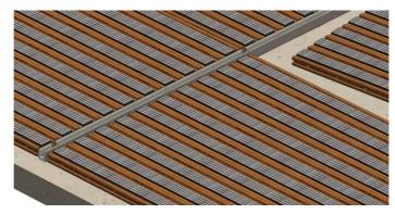
The base profile should be screwed to the floor using plugs and screws (not provided), the base profile is pre-drilled to aid this process. It is important to carefully mark the drill points on the floor ensuring the drill points correspond with the holes in the pre-drilled base profile and all base profiles are running straight. Insert the floor plugs first and then place the base profile on top and screw to the floor (see image above).
