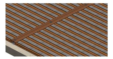
The top profile can now be simply screwed into the base profile using a 4mm Allen key (not provided), the base profile has a location thread along its entire length, do not overtighten the top profile screws.
