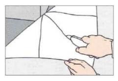
ii) To enable the material to bend more easily, the reverse side of the insert should be grooved to approximately half thickness of the material using a 'P' Type grooving tool.
