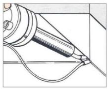
v) All exposed edges must be sealed with a sanitary sealant that is resistant to fungus and mould
