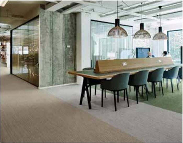
Tessera and Westbond carpet tiles: Tessera is available in 100% post-consumer recycled yarn, with a backing of 78% recycled and reused content. Westbond tiles have a recycled PVC backing.
