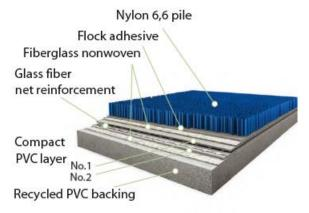
Figure 1: Typical construction
