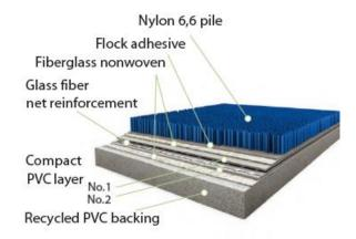
Figure 1: Typical construction
