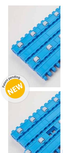
Based on series 8, the RTP A90 type offers a roller top (RTP) with rollers rotating at an angle of 90° to the conveying direction (A90). This guarantees products to slide onto and off the belt sideways with little friction.
