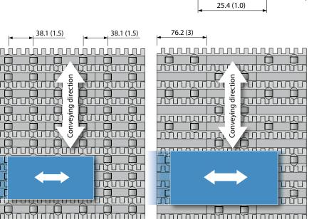
Roller top belts can be adapted perfectly to match the shape and weight of the products conveyed. Changes are easy to make.
